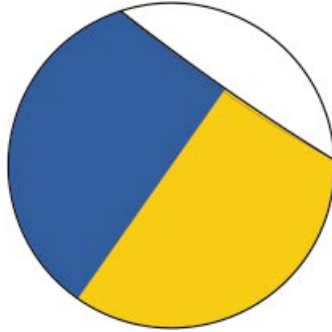
FIGURE 8. The granular material is initially divided into two regions of equal mass with one half shaded yellow and the other blue. All the particles are of the same size, surface roughness and density and differ only in their colour. The drum is rotated with constant angular velocity and the two regions mix during steady flow. The avalanche takes place in a thin layer close to the free surface. The interface between the avalanche and solid body region below it is shown by the thin black line.
